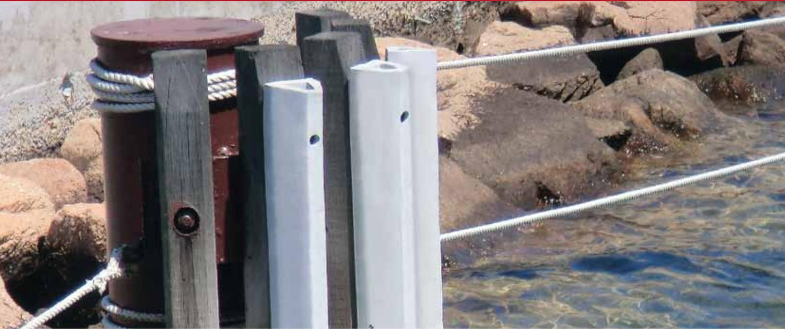
The delta fender is a proven effective rubber profile for use in both marine and industrial markets and they can be used for various purposes, both inside and outside. This type of fender has a minimal contact surface and they are easy to assemble. A properly mounted delta fender has the capacity to absorb high levels of energy through the presence of a relatively large hollow chamber.
